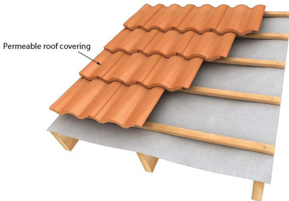
Figure 1: Cold Roof detail with permeable roof covering
